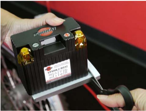
In this example, we only needed to shim the height. Do the same if the original battery is significantly larger in width or depth, and trim the selected spacers to fit with scissors.
