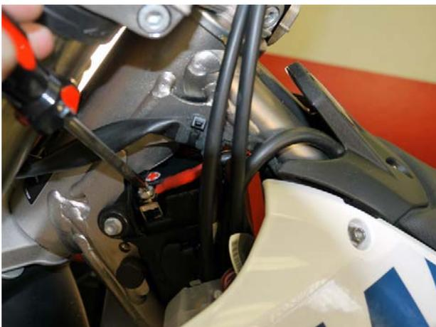
Max torque for the terminal screws is 30kg/cm (26 inch/pound). Do not over-tighten. We recommend the use of a #3 (big!) Phillips screwdriver, as this allows you to apply downward pressure on the terminal screw. That helps the threads catch, and reduces torque on the terminals. Note that the terminals are not anchored at back, and may twist slightly during install. If so, performance is not affected.
