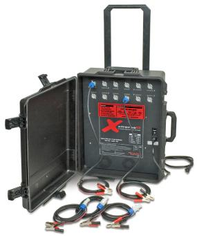
The Xtreme 12-Station Heavy Duty Battery Charger (SC-12) is a 12-station, 6 amp per channel, battery charger that recovers, charges and desulfates any type of 12-Volt lead acid battery. It uses universal electrical input and can operate anywhere in the world with a detachable IEC connector. Each of the twelve stations operate in isolation from one another allowing any combination of batteries, up to 12, to be recovered, charged and desulfated.
