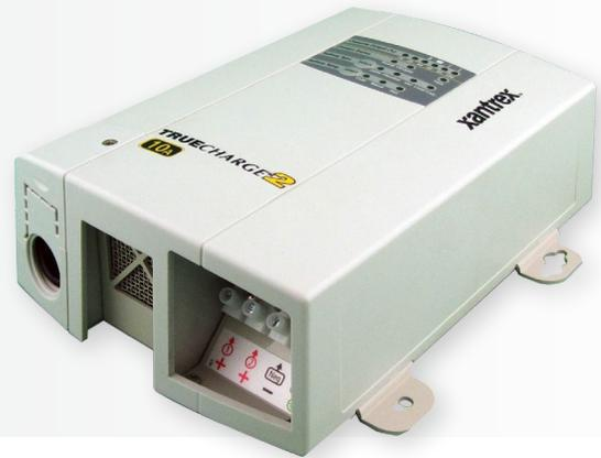
TRUECHARGE2 Battery Chargers lead the industry with a small footprint and ultra-compact design. Designed for marine and commercial applications worldwide, the TRUECHARGE2 10-amp replaces the former best-selling, first-generation TRUECHARGE 10TB unit and features universal auto ranging input voltage (90 Vac to 265 Vac, 47 to 63 Hz), which can be used in most parts of the world. The TRUECHARGE2 10-amp is smaller and lighter than its predecessor and can be mounted in a variety of positions.
