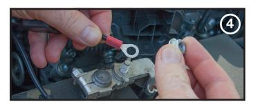
Connect the positive (+) wire to the positive (+) battery terminal. After removing the nut from the bolt securing the battery clamp to the positive terminal, slip the round metal lug at the end of the positive red SolarPulse wire onto the bolt until it sits next to the clamp.
