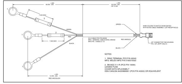
Cable to cranking battery
