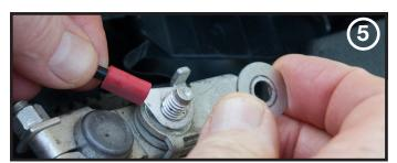
Slip a round washer (not included) onto the bolt until it sits next to the lug. Replace the nut onto the bolt and tighten it until it secures the lug and washer against the clamp. Do not over tighten. Repeat steps 4-5 above to connect the negative (-) black SolarPulse wire to the negative (-) battery terminal.
