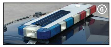
Mount the solar panel using any of the following methods: Four roundhead screws, industrial adhesive, heavy-duty dual lock or double-sided tape (not included). It should be mounted where it will have direct sunlight.
