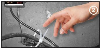
If needed, use plastic cable ties (not included) to secure the circuit box wires to the battery cable or other secure area near the battery. This will keep the wires from being damaged or interfering with any moving engine parts.
