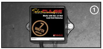
The circuit box can be mounted using any of the following methods: Two round-head screws, industrial adhesive, heavy-duty dual lock or double-sided tape (not included). After cleaning the install area, mount the box close to the battery so that the lugs can reach the terminals. DO NOT attach it to the battery itself. Also make sure the box is located in a location where it won't be disturbed and the LED is visible.
