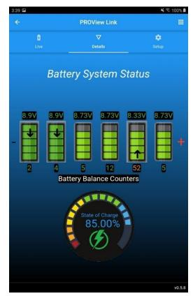
Counters under each battery will represent how many times a battery has been balanced. Red, Yellow, or Green numbers are visual aids to show which battery was balanced more/less than the other batteries in the pack. A Red number may indicate that specific battery is the weakest (weak link) in the pack while a Green number may indicate the strongest battery in the pack.
