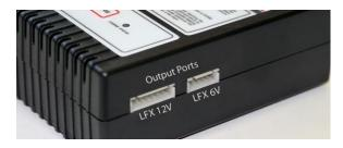
At this point you should have the battery charge cable connected to the battery BMS port, and the AC input cord connected to the charger. Now insert the AC plug into an appropriate AC wall socket. Whenever possible, use the charger's retractable hook to hang the BMS01 above the floor, in a location which allows easy access to the battery charge cable. Now plug the battery charge cable into the correct LFX<sup>TM</sup> charge output port (or into the extension cable).
