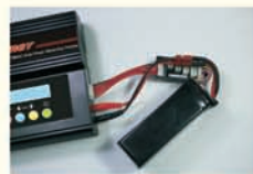
connection diagram in the balance charging /storage/discharge mode
