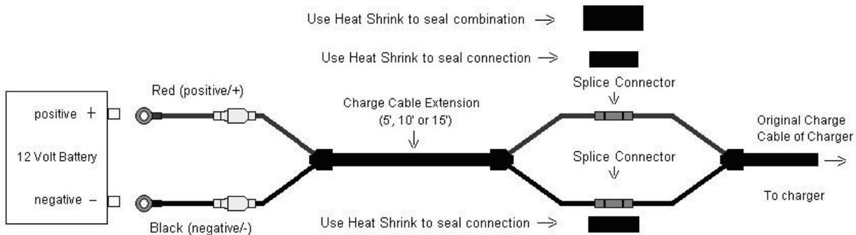
To connect the charger to the battery (batteries), route your charge cables from the charger to the batteries, being cautious to avoid sharp objects, and use the supplied wire ties to hold them securely and neatly in place.
