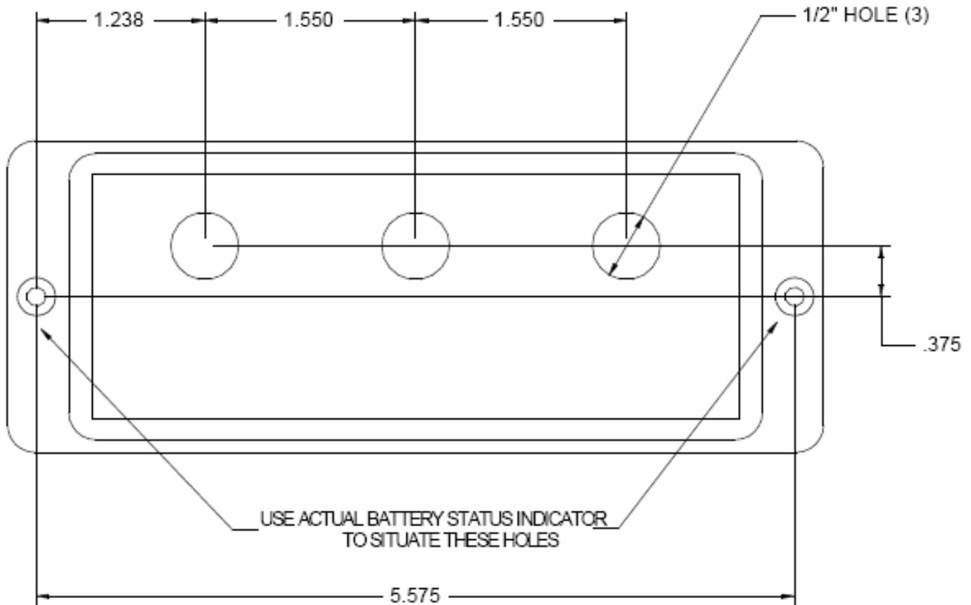
1. Locate remote indicator template at desired location. Drill a pilot hole at the center of each hole position using a 1/8" bit. Once the pilot holes are ready, drill three 1/2" holes where indicated. Care should be taken to thoroughly clean the surface with isopropyl alcohol after the holes have been drilled.
