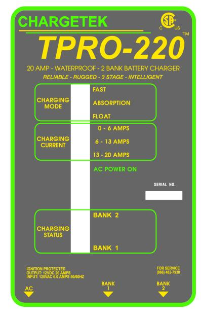
indicated by the AC Power On and Fast LEDs flashing. If the over voltage persists then the factory should be consulted.
