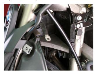
The LFX batteries can bolt cable eyelets to either the top or front sides of the terminals. **Be sure to Install the POSITIVE terminal cable first**, then Negative, to avoid short circuits.
